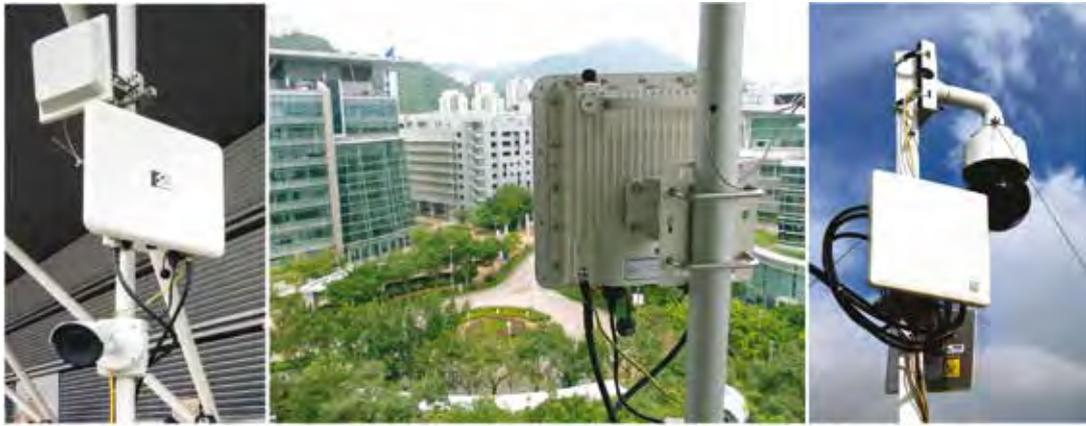
Left: P2 X30 MeshRanger with AXIS P1428-E (4K ultra HD surveillance), Center: P2 X30 MeshRanger
